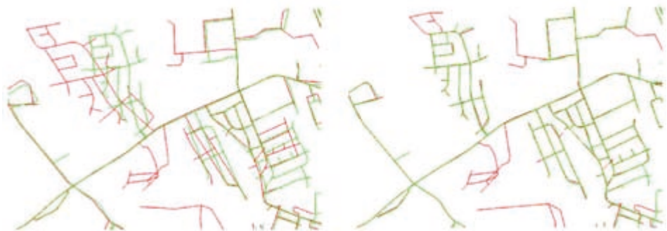
Figure 13: A conflation process – two original datasets (left) and the conflated overlaying result (right). (Source: Gabbay, 2004)
