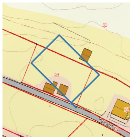
Figure 3. Result of Experiment 1 (direct elicitation). GPT-5 polygon for parcel 12/38 shown in blue; cadastral map boundary in red. The protrusion to the southeast arises from the model's attempt to close the polygon without violating the measurements and bearings given in the skyldskifte .
