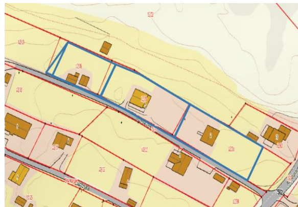
Figure 5. Result of Experiment 3 (anchor revised to south-west corner). GPT-5 boundary proposals (blue) for the Gnr. 12 cluster; cadastral map boundaries in red. The cluster geometry aligns more closely with the road and fence lines.
