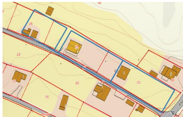
Figure 4. Result of Experiment 2 (relational reasoning, single south-east anchor). GPT-5 polygons for parcels 12/38, 12/20 and 12/21 in blue; cadastral map boundaries in red. Residual discrepancies are attributable to an inconsistency between the source documents and the choice of anchor point.
