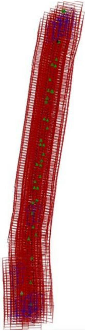
Figure 12: Image Footprint for 4 flights including Nadir and Oblique Camera footage and Check point locations
