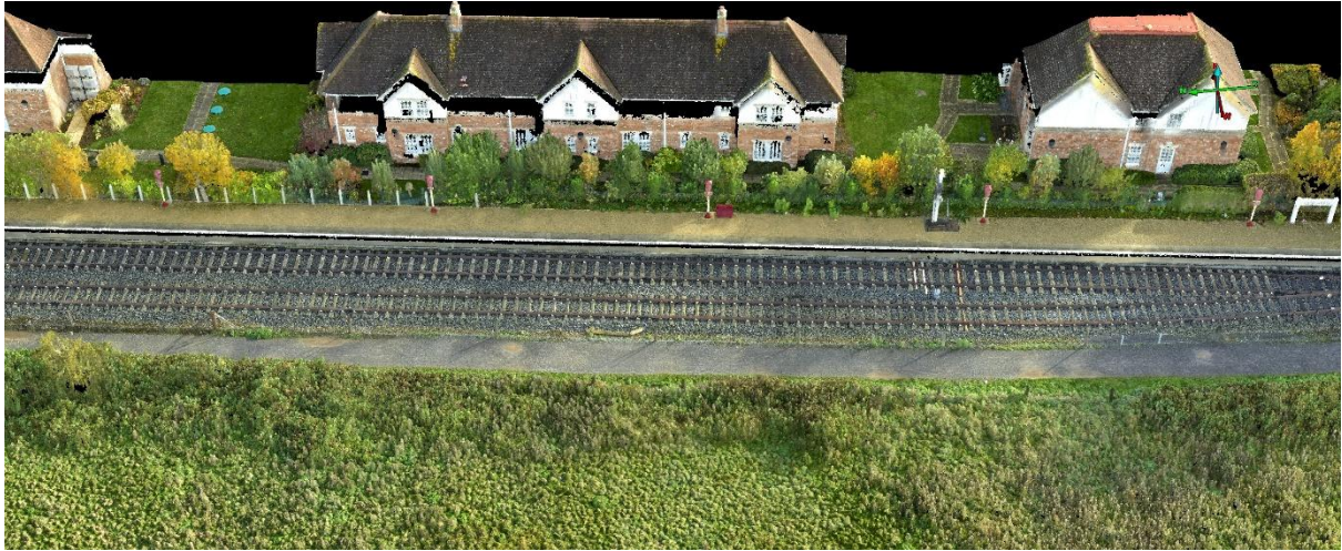
Figure 13: Colorized Photogrammetric Point Cloud
