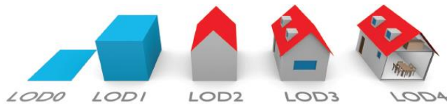
Figure 2. Increasing Levels of Detail in CityGML (Rajabifard et. 2019)
