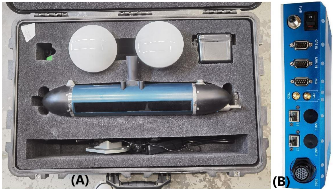
Figure 1. (A) 3DSS-IDX-450 Sonar with GNSS. (B) Sonar Interface Unit (SIU) powers the sonar head and has an integrated Ethernet switch for communication with the sonar head (Ping DSP Inc., 2021).
