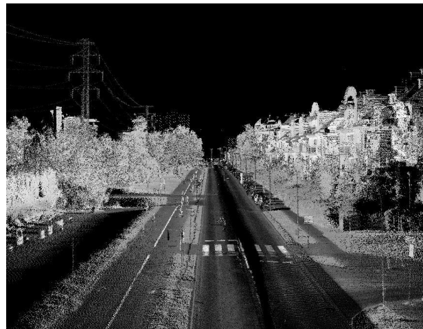
Figure 3. Students' work: the visualisations of the acquired point cloud from laser scanning (TLS and MLS).
