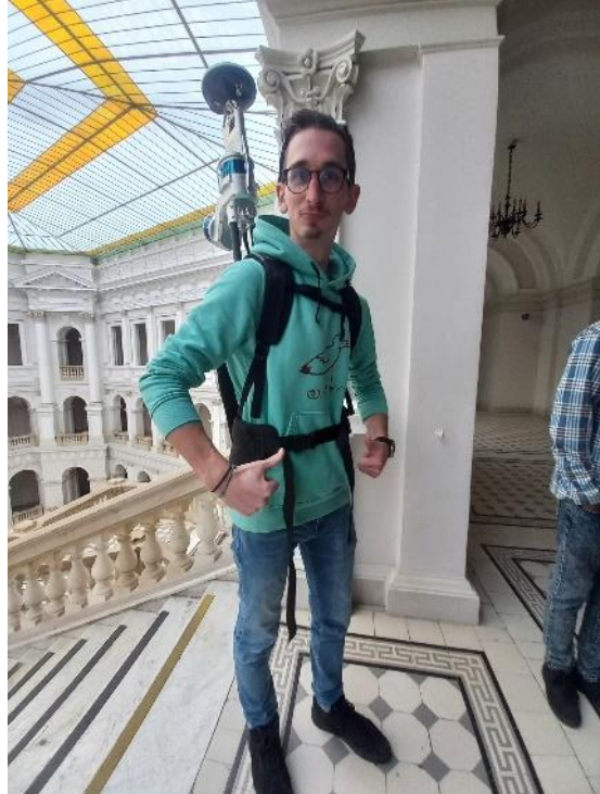
Figure 2. Students work on the measurement using terrestrial laser scanner and mobile scanning backpack
