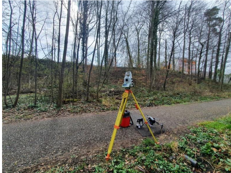
Figure 6: Free station using the stop and go method
