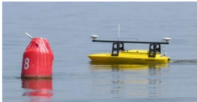
Echoboat R/c hydrographic survey USV. Courtesy NOAA
