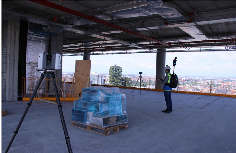
Figure 6: The mapping activity with HERON and Leica RTC360
