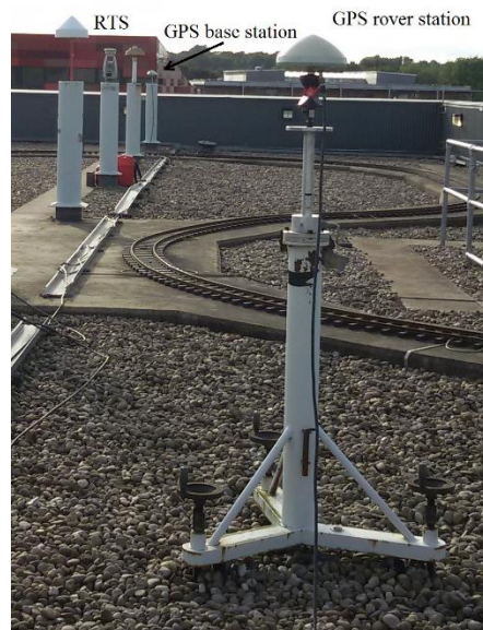
Figure 2. Experiment set-up consisting of the GPS antenna and the 360° prism mounted on a heavy-duty tripod, the GPS reference station and the RTS.
