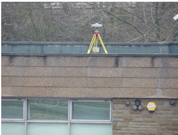
Figure 3. The principal reference GNSS antenna located upon an adjacent building to the
