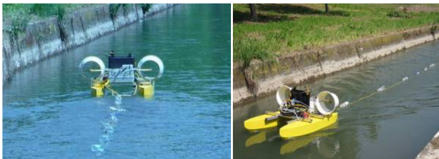
The aerRobotix CatOne robot boat tows the electrode array during tests in a canal.
