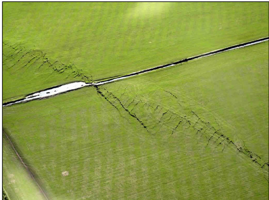
Figure 3: A section of the Darfield earthquake fault rupture showing the complexity of the local deformation across the trace. (GNS Science geologists Richard Jongens, Simon Cox and David Barrell)
