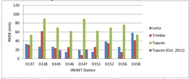
**Fig. 10**: Height RMSE test with c. 45 minutes observing time and GLONASS not included. Note Topcon heights shown in green were subject to an incorrect receiver setting.
