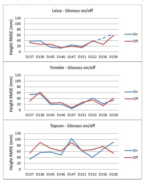
Fig. 11: The effect of including/excluding GLONASS in the each manufacturer's height solution.
