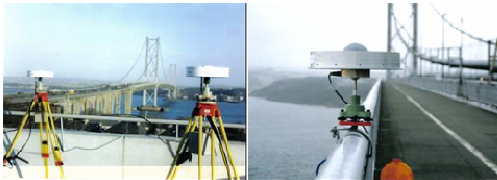
Figure 10. Two GPS reference receivers located adjacent to the Forth road bridge (left). A GPS choke ring antenna attached to the bridge (right).
