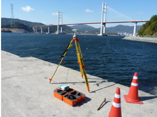
Figure 16. One of the reference GPS receivers adjacent to the Pusan Bridge
