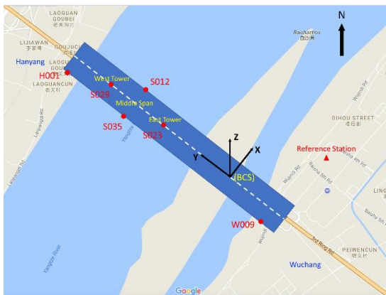
Figure 4. Monitoring stations set-up on the bridge (The background figure is from Google Earth). A Bridge Coordinate System (BCS) was defined by this paper (X and Y denotes to lateral and longitudinal direction of the bridge, and Z is orthogonal with the plane of X and Y and denotes to the height direction).
