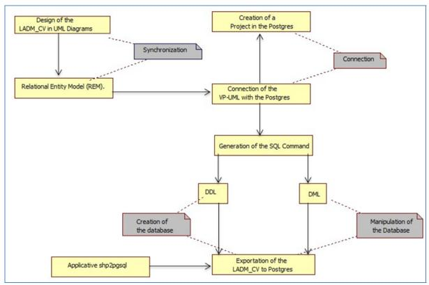
Figure 5. Flowchart showing the specification of the LADM\_CV in a relational database
