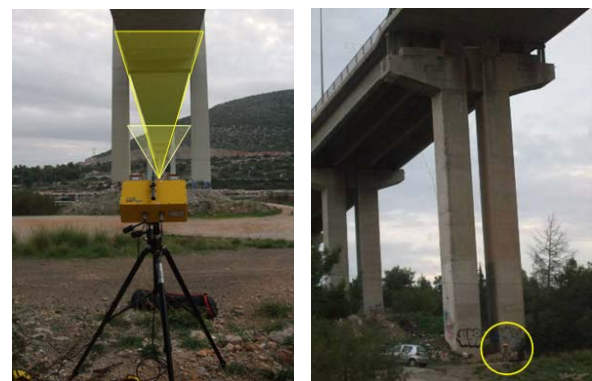
Figure 4. IBIS-S system setup. The triangles in yellow denote the area of observation (left), whereas, the circle denotes the location of the instrument by the basement of the pylons (right).
