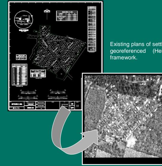
Existing plans of settlements can be identified in the field and be georeferenced (Helmert-transformation) to the reference framework.
