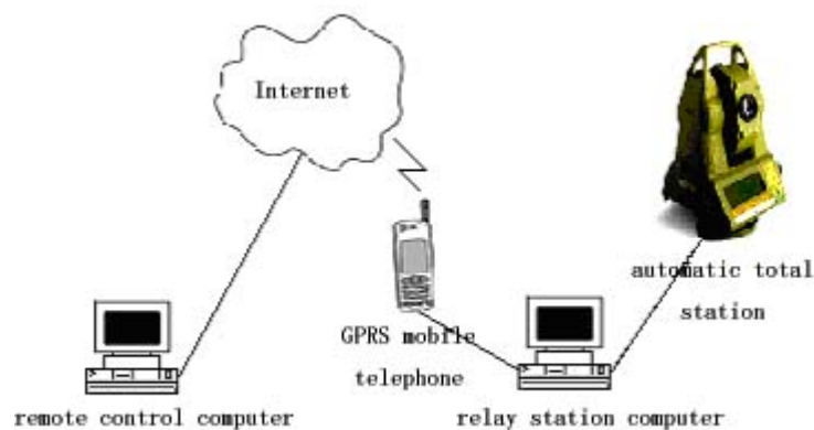
Figure 2: Wireless communication based on GPRS
