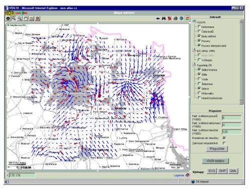
Figure 2: Resulting interpolated movements of Ostrava network
