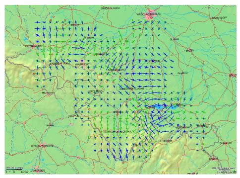
Figure 6: Resulting deformation field
