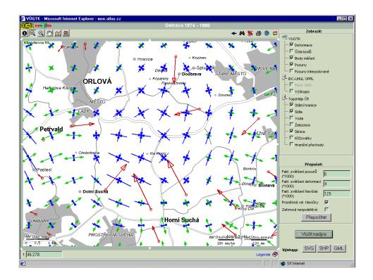
Figure 3: Outline with given displacements and determined deformations of Ostrava network
