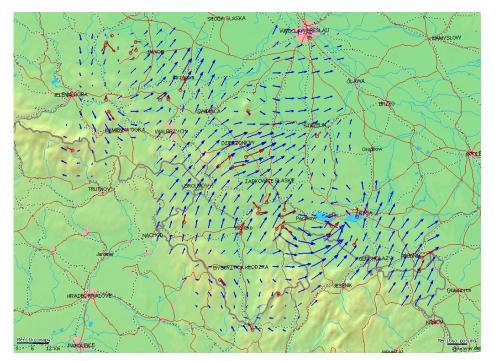
Figure 5: "Local" displacements after reduction using tectonic plate motion model
