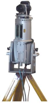
Figure 1: Nikon D 100 mounted on top of LMS-Z420i
