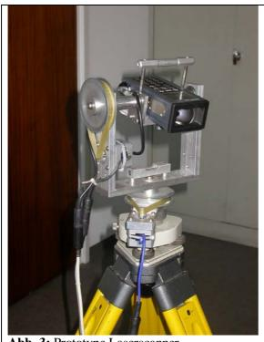
Abb. 3: Prototype Laserscanner
