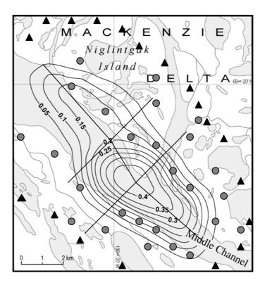
**Figure 1:** Detail of the Niglintgak Island area showing the predicted subsidence bowl (contours in metres), the spread of monuments in Model A (circles) and the artificial monuments (triangles), and the major axes of the subsidence bowl
