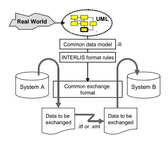
Figure 1: Data transfer between different information systems through a common data model defined through a common data description language.
