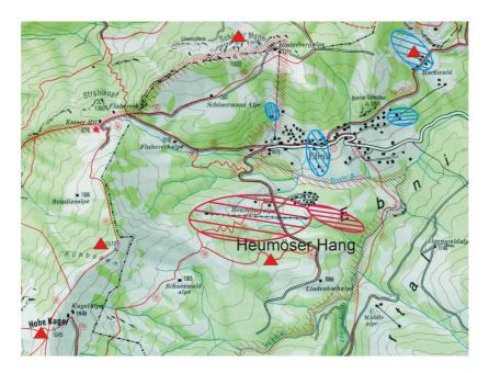
Fig. 1 Deformation network Ebnit with the reference points (triangle) and the 5 examination areas ("Heumöser Hang" red)
