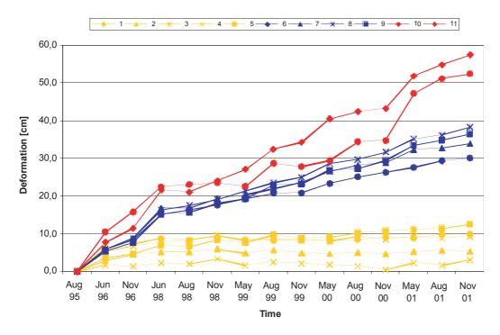
Fig. 4 Deformation analysis "Heumöser Hang" points 1-11, all epochs, horizontal displacements
