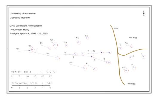
Fig. 5 Deformation analysis "Heumöser Hang" 4<sup>th</sup> and 15<sup>th</sup> epoch, points 1-11 and 50-62, horizontal displacement vectors with their confidence ellipses
