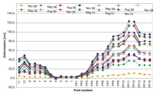
Fig. 6 Horizontal deformation characteristics of "Heumöser Hang", 14 epochs, GPS points (1-11) and the traverse
