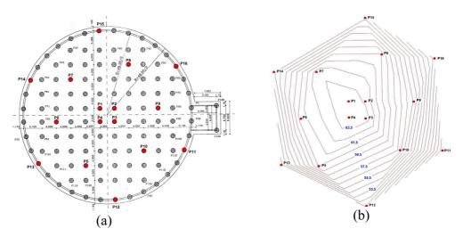
Fig. 9. Layout of foundation piles (a) and measured vertical displacements (b) of the 50,000 t sugar storage tank at Plati
