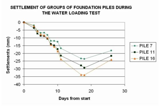
Fig. 5. Settlement of pile 7 (external periphery of slab), 11 (intermediate periphery), and 16 (center of slab)
