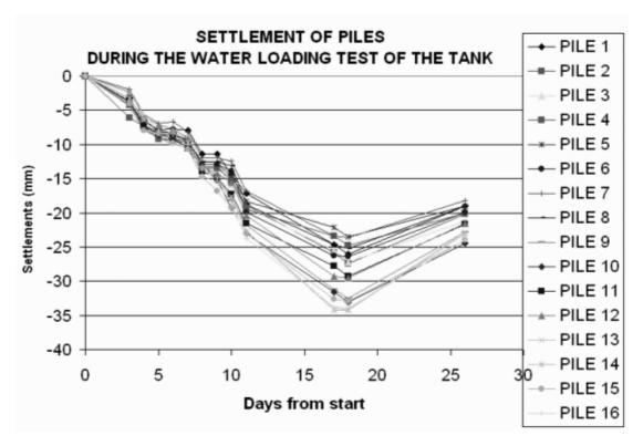
Fig. 4. Settlements of all piles during the water loading test of the tank in June, 1983
