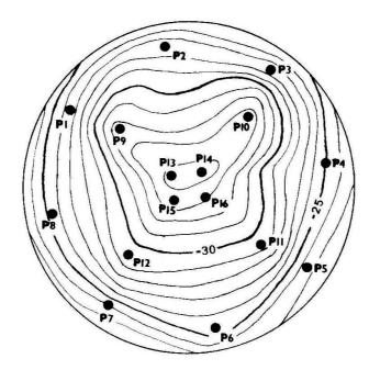
Fig. 6. Lines of equal vertical displacement of piles under maximum load during the water loading test of the tank
