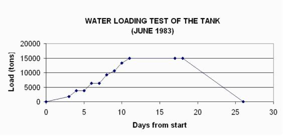
Fig. 3. The water loading test of the liquid ammonia tank in June, 1983
