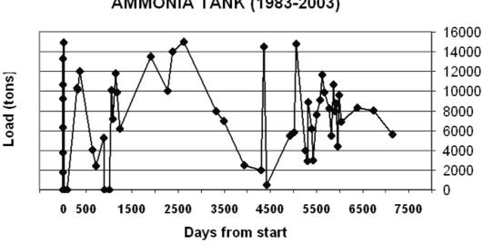
Fig. 7. Total loading history of the liquid ammonia storage tank (1983 – 2003)
