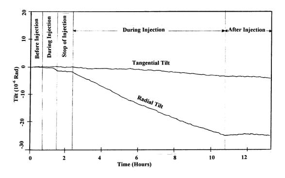
Fig. 1. Typical tilt signals recorded by station No. 9
