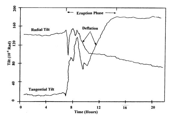
Fig. 3. Tilt curves observed during an eruption
