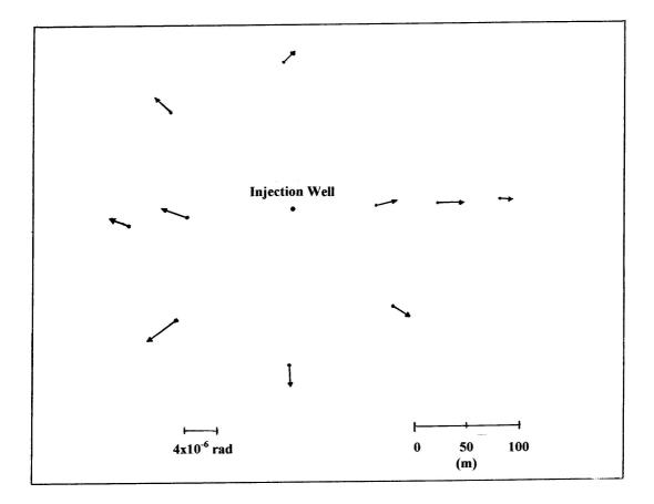
Fig. 2. Tilt vectors observed at different tiltmeter stations
