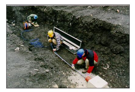
Figure 7. Measurement using the hydrostatic profile gauge (the probe is being pushed)
