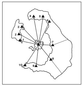
Figure 2: Baselines for the volcano geodetic monitoring EDM network.
