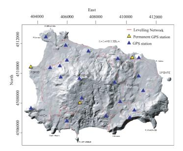
Fig. 14- GPS and levelling networks operating on Ischia Island
