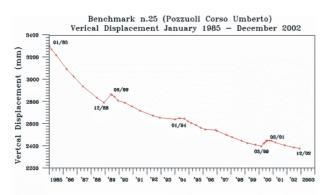
Fig. 8- Vertical displacements vs time at benchmark 25, located near to maximum uplift area, during the period 1985-2002.
