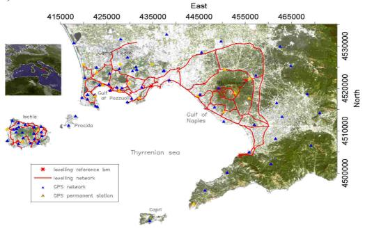
Fig. 1- GPS and levelling networks operating on the Neapolitan Volcanic Area.
