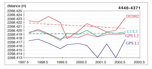
Fig. 3. Comparison GPS and EDM derived distances
