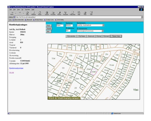
Figure 3. The Danish cadastral information system on the Internet. The textual information is presented on the left side of the screen by pointing on the relevant property (circled) in the map or by asking for this property by cadastral number or address. Zoom facilities etc. is available as well.
