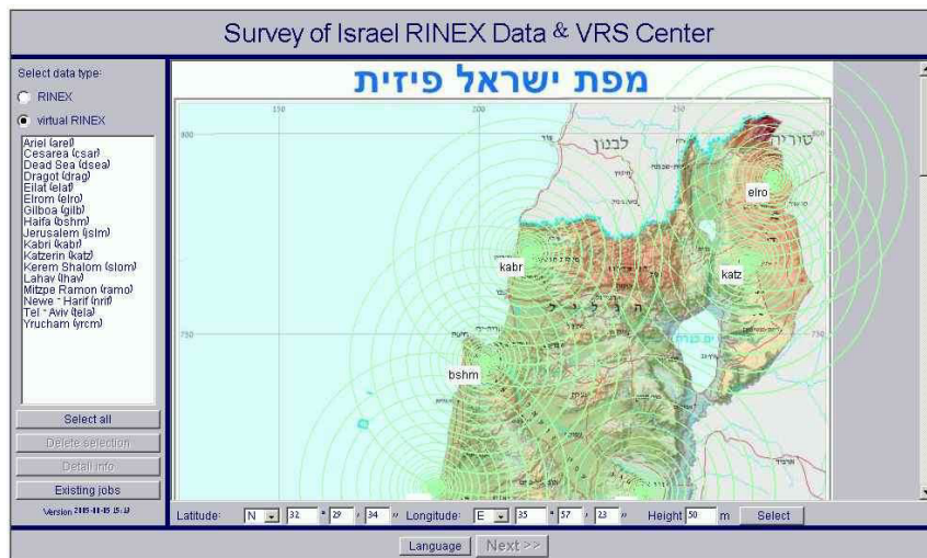
Figure 4. The internet GN_web module in web (www.mapigps.co.il) enables users to ask for a permanent station data or a user defined VRS station data within the APN.
