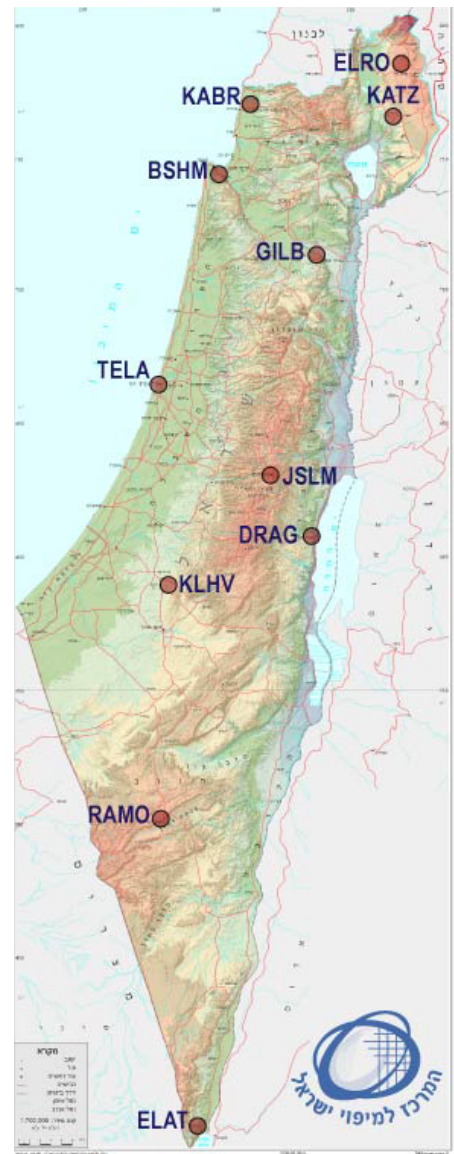
Figure 1. The GIL reference stations at the completion of the combined effort between IGS, Israeli Space Agency, The Survey of Israel and Tel-Aviv University on 2002.
