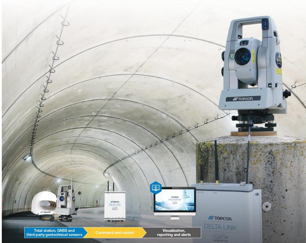
**Delta Solutions: Complete autonomous monitoring solutions** – Topcon's Delta hardware and Software solutions provide a complete data set for a thorough understanding of focused assets for deformation monitoring.
